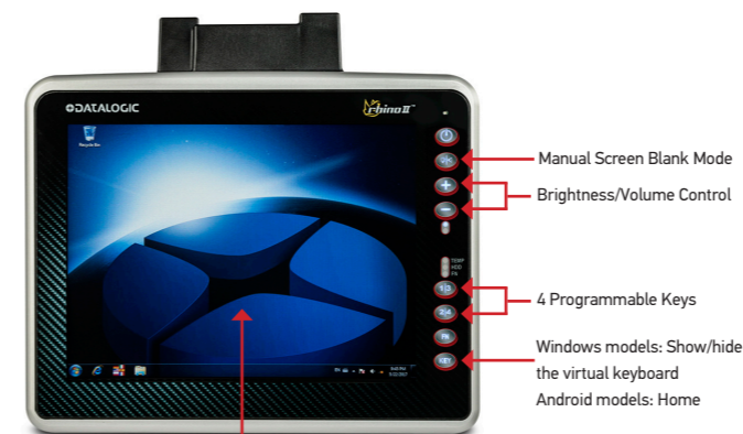
Capacitive Touch Display 3 mm non-reflecting armored glass
