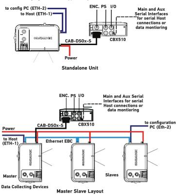
After making system cabling, connect a compatible device to the CBX510's 25-pin Device Connector through a proper cable. Power on the compatible device. The CBX510 Power LED turns on (blue) when the power connection has the correct polarity. In case of wrong polarity, no power is passed to the CBX510 and the Power LED remains off.
